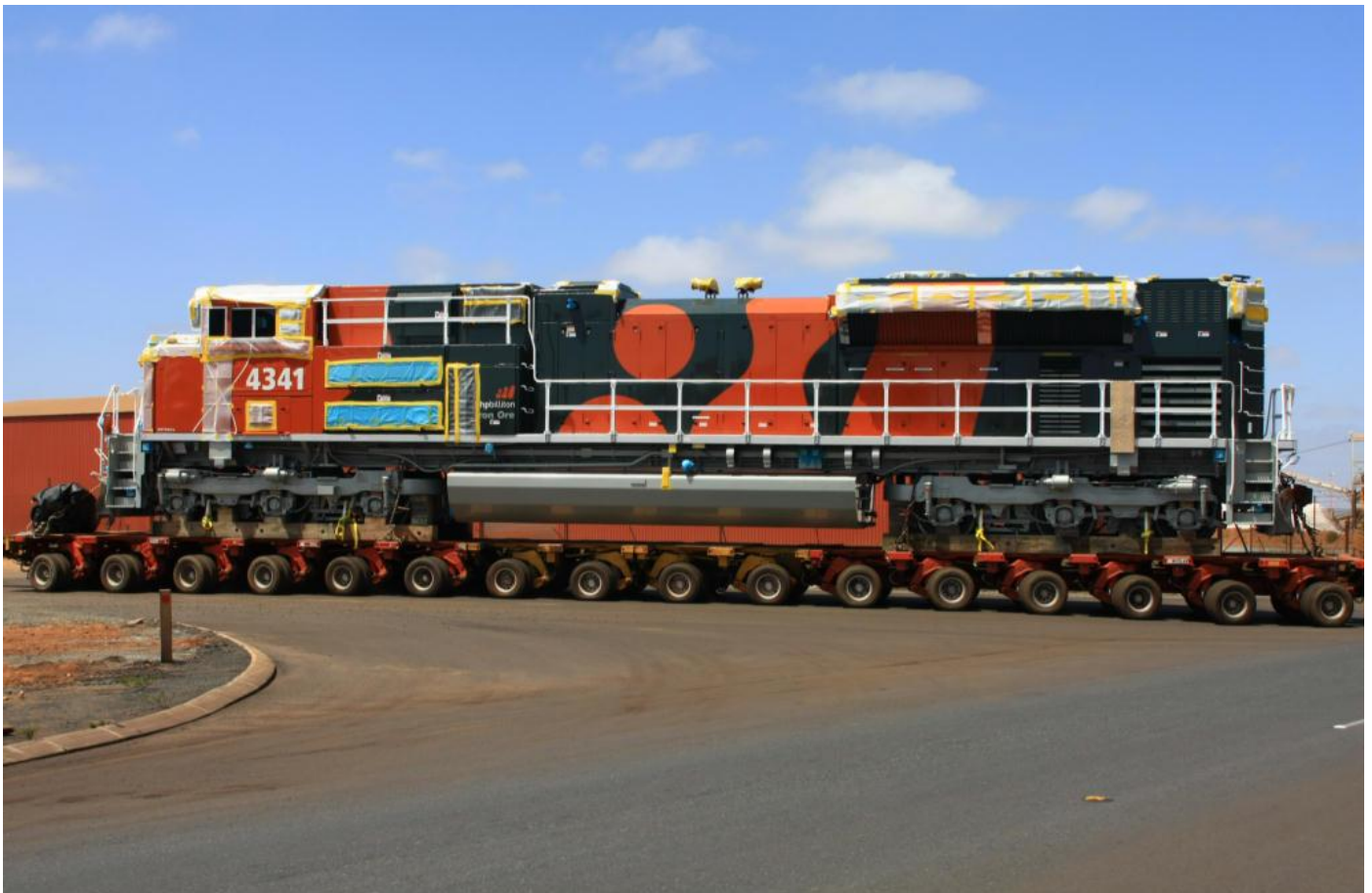
Side on shot of 4341 as it turns off Gilbert Street and enters the Nelson Point complex through gate #9 on January 14th note wooden brackets under bogies allowing locomotives to be shipped complete. Photo Toad Montgomery
