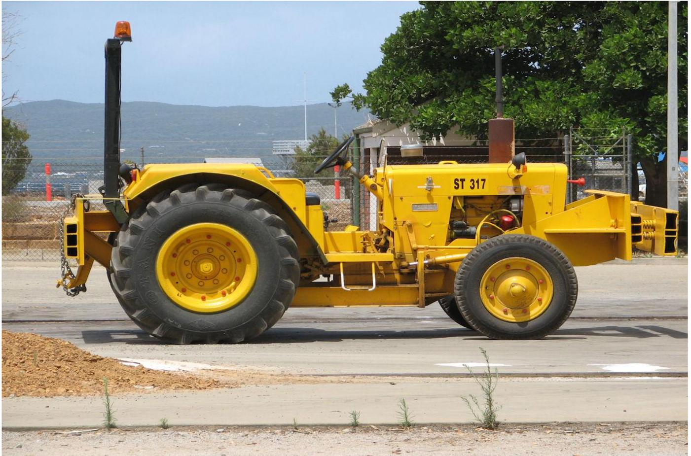
ST317 an old Mk11 Chamberlain tractor is now Albany's shunting tractor it's being used to move wagons around the repair depot was stabled outside Albany workshop on February 11th. Photo Stew Winston
